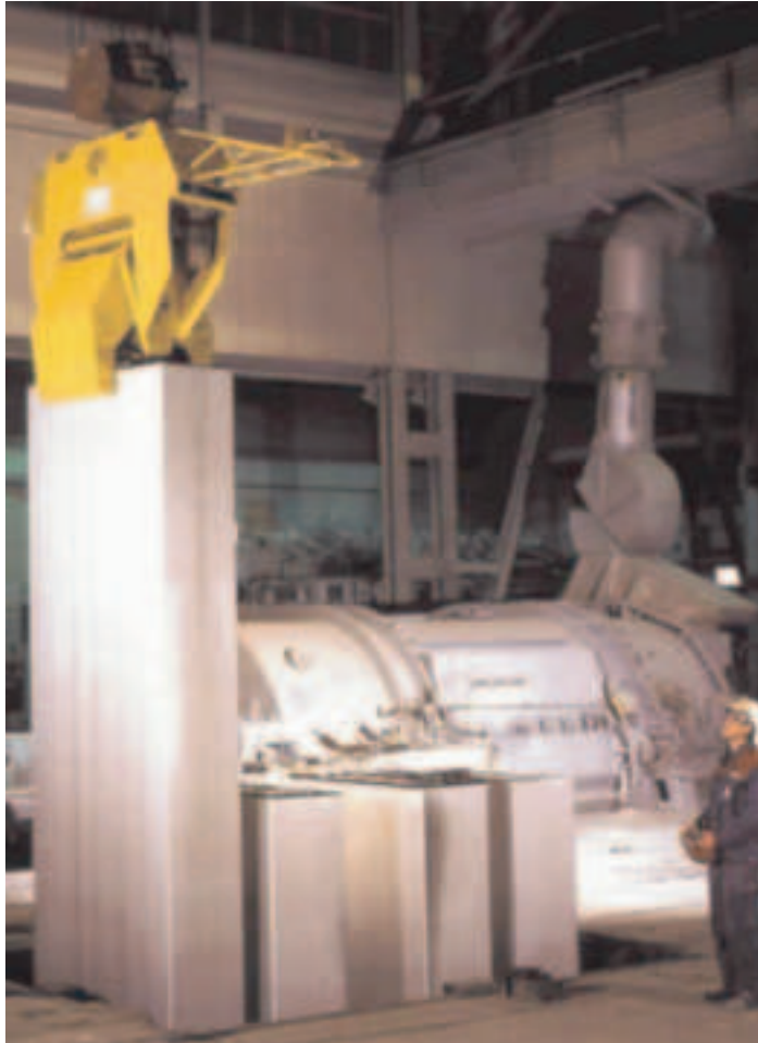
Figure 1: Sheet ingot cast at Hydro Aluminium Årdal, Norway. The cast weighs 13 tons and is worth about NOK 170.000. The picture is taken from the annual report of SINTEF Materials Technology, 1998.
